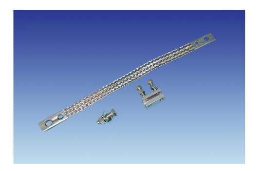
**APPLICATION:** Includes flexible stainless steel strap and bonding hardware to bond the thief hatch lid to mounting collar reducing the potential for electrical arcing in flammable environments on steel tanks.
