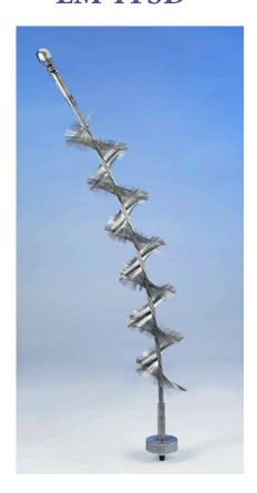
**APPLICATION:** The ITSD employs the point-discharge principle to neutralize the build-up of static charge, and to equalize it to the potential of the bonded mass of production, frac flow-back, or storage tank, reducing the likelihood of arcing. ITSD's are hardened to withstand the rigors of a sour gas (high H2S, chlorides, and mineral acids) environment. We accomplish this with a combination of cathodic protection and the use of alloys specifically designed for use in this environment.
