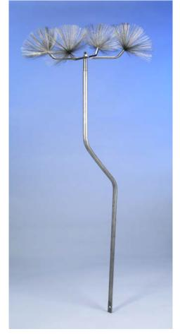
**APPLICATION:** For use wherever an air terminal (lightning rod) is appropriate and streamer delaying, or static dissipating qualities are desired. These air terminals are used in place of standard air terminals in a structural lightning protection system installed to UL-96A and NFPA 780 specifications. Terminal is mounted to the base most suitable to the structure on which it is being installed.
