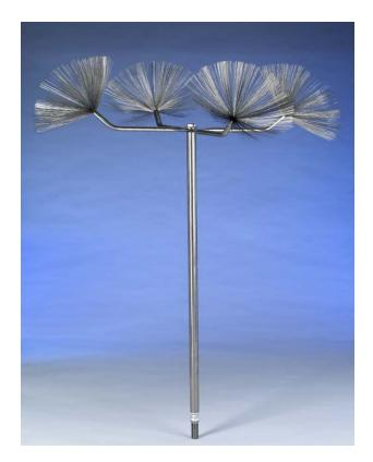
**APPLICATION:** For use wherever an air terminal (lightning rod) is appropriate and streamer delaying, or static dissipating qualities are desired. These air terminals are used in place of standard air terminals in a structural lightning protection system installed to UL-96A and NFPA 780 specifications. Terminal is mounted to the base most suitable to the structure on which it is being installed.
