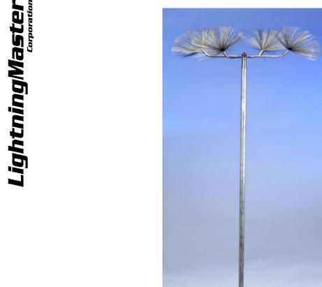
**APPLICATION:** For use wherever an air terminal (lightning rod) is appropriate and streamer delaying, or static dissipating qualities are desired. These air terminals are used in place of standard air terminals in a structural lightning protection system installed to UL-96A and NFPA 780 specifications. Terminal is mounted to the base most suitable to the structure on which it is being installed.
