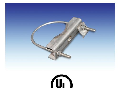
**APPLICATION:** UL listed stainless steel u-bolt bonding clamp provide 1-1/2" of surface contact on pipe with cable clip. Use with class I & class II lightning protection conductors.
