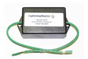
The Ground Wire Filter™ (GWF) effectively eliminates "sneak path" transients from entering sensitive electronic equipment through the ground wire. The GWF is a specially designed and wound toroidal choke/filter that presents an extremely high impedance path to high frequency transients. It absorbs and blocks their passage along the ground wire feeding into your sensitive electronics equipment, reducing downtime and damage.
