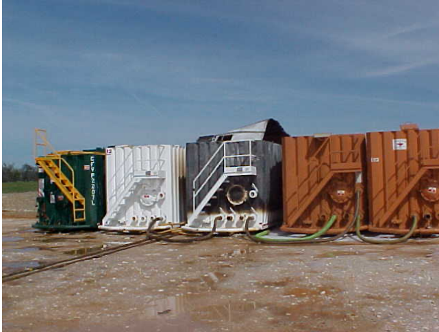
Damage to closed flowback tank caused by static ignition
