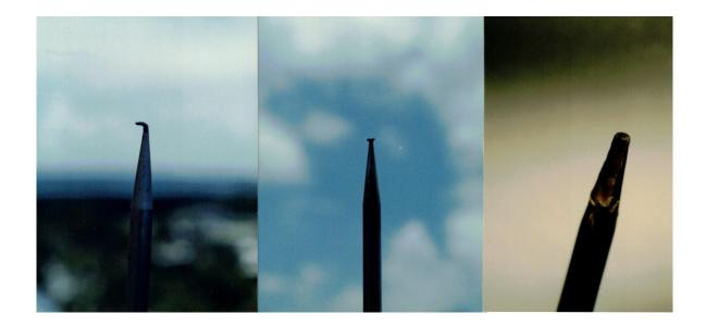
Conclusion. Applying the just barely molten principle of thermodynamics, it is apparent that not only is a Lightning Master Ultra-Sharp Point<sup>™</sup> air terminal unlikely to cause a fire, but that a Franklin lightning rod is actually more likely to cause a fire.
