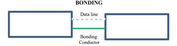
Grounding is a matter of bringing the bonded equipment mass to the potential of the surface of the earth which it occupies. Again, the primary reason is personnel safety, and the secondary reason is equipment protection. When it comes to grounding, we need to consider two types of grounding: low-impedance grounding of structures, and single-point ground potential referencing for services and equipment.
