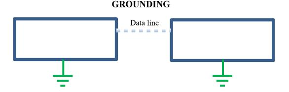
If equipment is grounded as shown above, any difference in ground potential between the equipment will be equalized through the data line, causing unwanted current flow and equipment damage.
