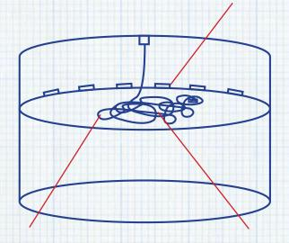
Loose cable can create a high-impedance path for current, increasing the risk for arching Cable can tangle and break, eliminating the electrical connection
