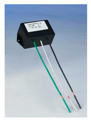
**APPLICATION:** The LM-HW-24V-S is a surge suppressor designed for 24 VDC applications in commercial and industrial process control and battery charging systems. It installs in parallel with the equipment and protects the connected devices from damaging overvoltage transients thus reducing equipment dmage and downtime.
