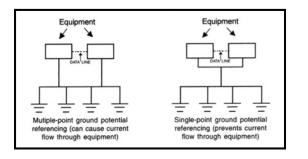
When we refer to the facility equipment, it is important to note that we are referring only to electrical or electronic equipment, not door frames, air conditioning ducting, miscellaneous masses of inductance, etc.
