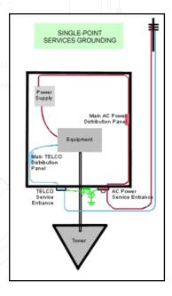
and equipment bonding sub-system to the grounding system.
