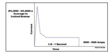
instantly. The surrounding ground charge rushes toward the point of the strike. If that in-rush of charge crosses a gap, it may arc. If that gap is between the floating roof and the side of the tank shell, and there are flammable vapors present, those vapors may ignite.
